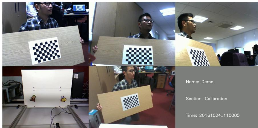
**Figure 3: An example of the Kinect-Camera calibration data**
