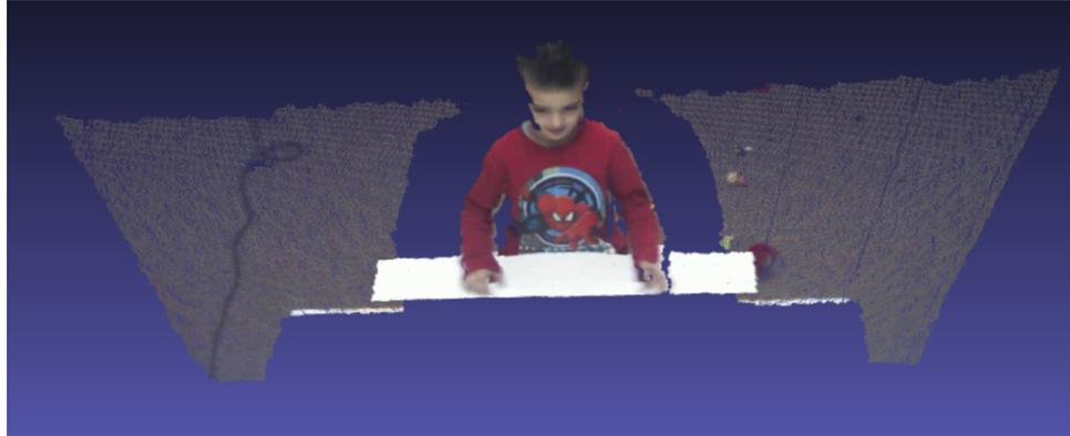
**Figure 4: The point cloud collection by a Kinect after the RGB image and the Depth image has been aligned. The Kinect is in front of the child.**
