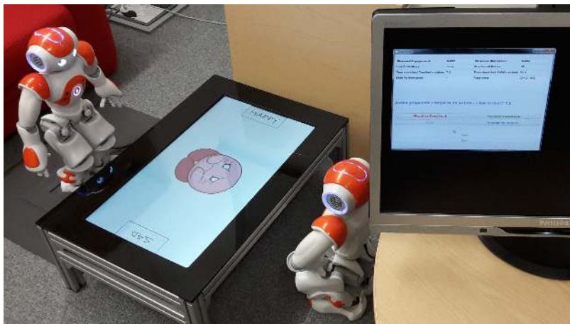
Figure 14: Setup used for the user study from the perspective of the human supervisor. The child-robot (left) stands across the touchscreen (centre-left) from the wizarded-robot (centre-right). The supervisor can oversee the actions of the wizarded-robot through the GUI and intervene if necessary ( right ).
