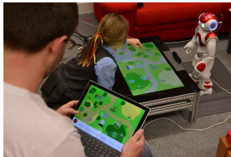
Figure 1. Interaction setup: the teacher (one of the authors) on the left uses a GUI on a tablet to control and teach the robot how to interact with the child until reaching a good action policy.
