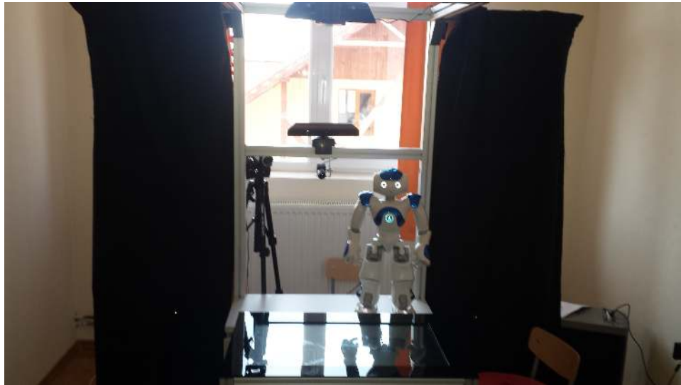
Figure 1: The final setup of the Sandtray with robot shown with the intervention table. The robot should ideally be centred in front of the screen to facilitate the interaction, and to ensure that the pointing behaviours are accurate.
