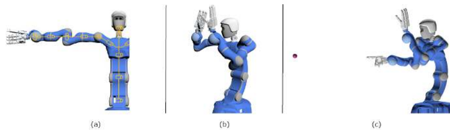
Figure 11: Example illustrating the calculation of a blended gesture for Justin. (a) Joint configuration of the robot. (b) Calculated end posture for the emotional expression of fear. (c) Calculated end posture for a combination of a pointing gesture with the right arm, accompanied by gazing towards the pointing location, and the emotional expression of disgust.
