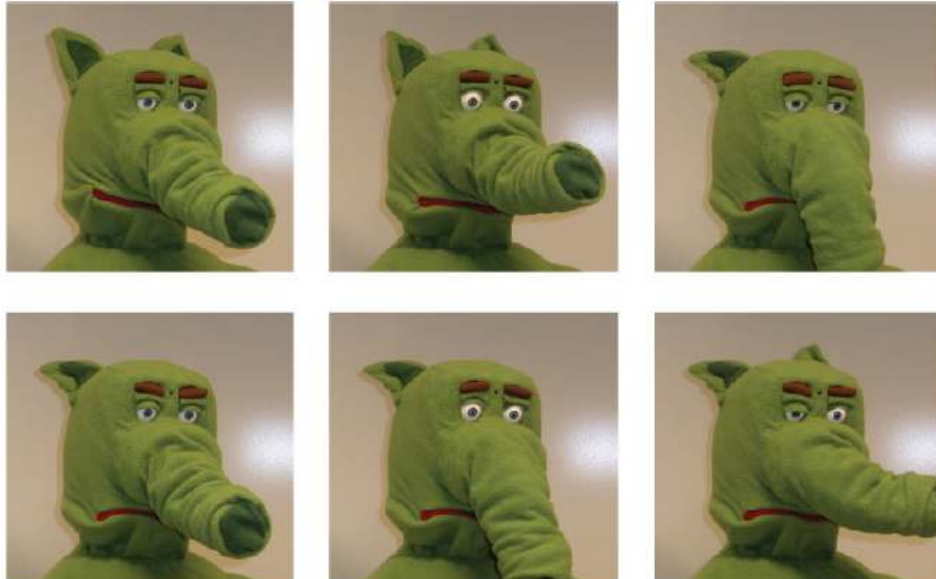
Figure 5: FACS has already been implemented in the huggable robot Probo to express different emotions.
