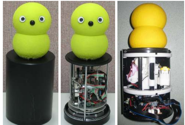
Fig. 1: Internal and external structures of Keepon Pro [9] and My Keepon.
