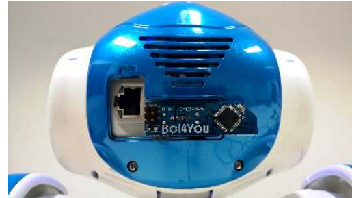
(b) The NAO eyebrows PCB is plugged into the USB port behind the head of the robot.
