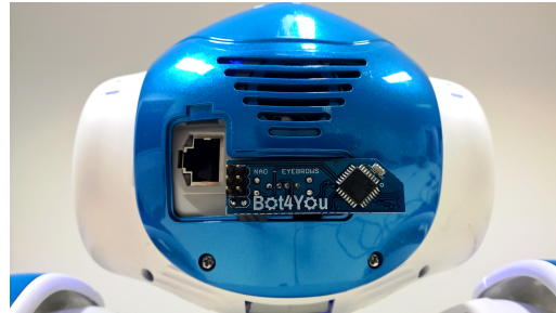
(b) The NAO eyebrows PCB is plugged into the USB port behind the head of the robot.
