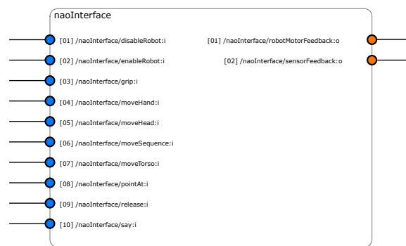
Figure 16: NaoInterface component yarp ports: the prefix for the port names is listed in the main text. This component is responsible to convert primitive into motor or actuator commands.
