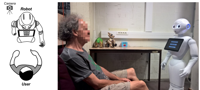
Fig. 11. The experimental setup in the elderly care scenario. A senior user plays a music game with Pepper robot.
