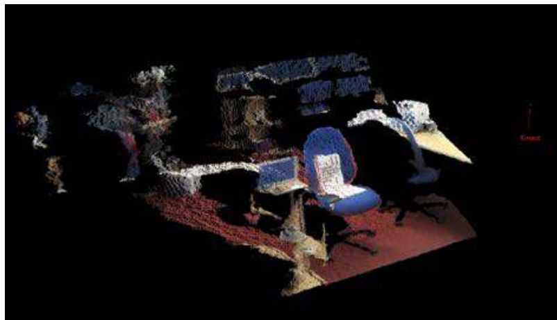
Fig. 6. The point cloud collection by a Kinect after the RGB image and the Depth image has been aligned. The Kinect is in front of the chair.
