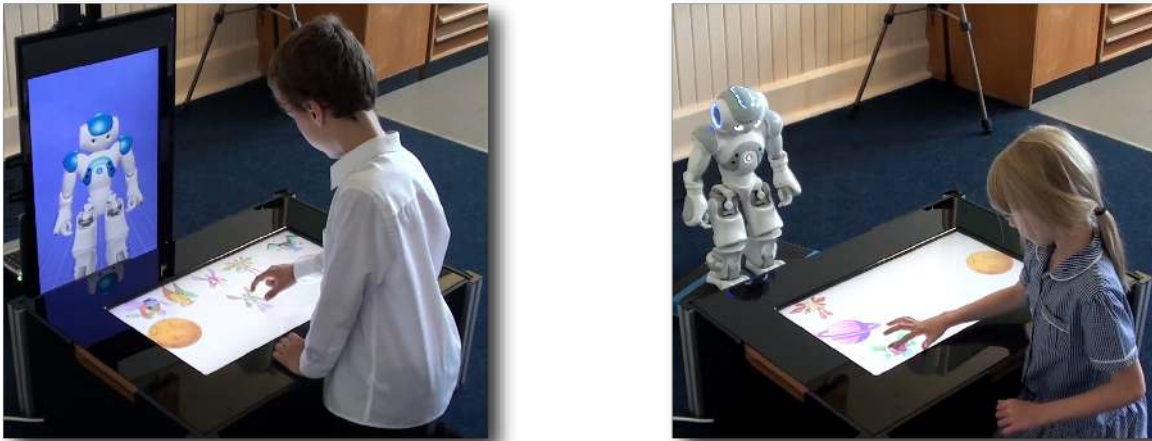
Fig. 1 Side-by-side images of the virtual (left) and real (right) robots used for this study: the Aldebaran NAO. The images are stills taken from one of the cameras used for filming. Scaling has been kept consistent between the two images so that size comparisons can be made.
