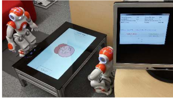
Fig. 1. Setup used for the user study from the perspective of the human supervisor. The child-robot (left) stands across the touchscreen (centre-left) from the wizarded-robot (centre-right). The supervisor can oversee the actions of the wizarded-robot through the GUI and intervene if necessary (right).
